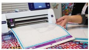
$step\ 6.$  Remove the heart shape (and remaining material) from the mat.
