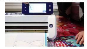
Place adhesive-backed magnet sheet with the magnet side facing down onto the mat. Select "Load Mat" > "Scan".
