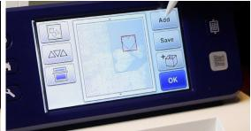
**step 4.** Using the Deep Cut Blade, perform a test cut. (Settings of "Cut Speed": 1 and "Cut Pressure": 5 were used.)
